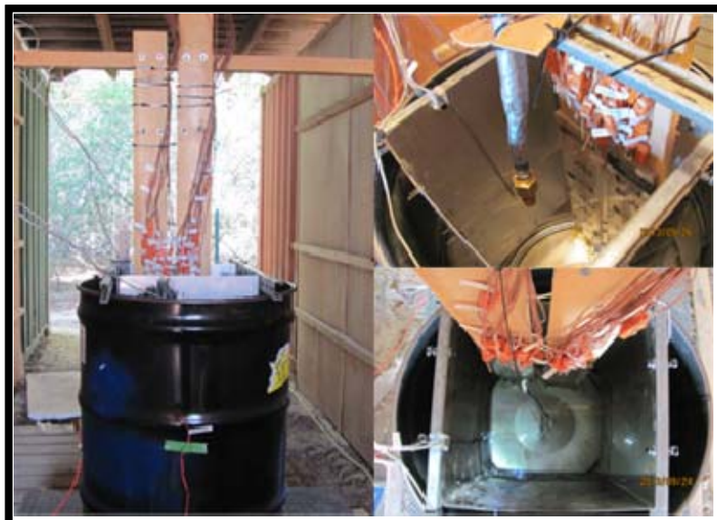
Experimental setup for release of LN 2 on water
