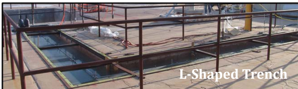
LNG release in L-Shaped Trench, Release duration – 1200 s
