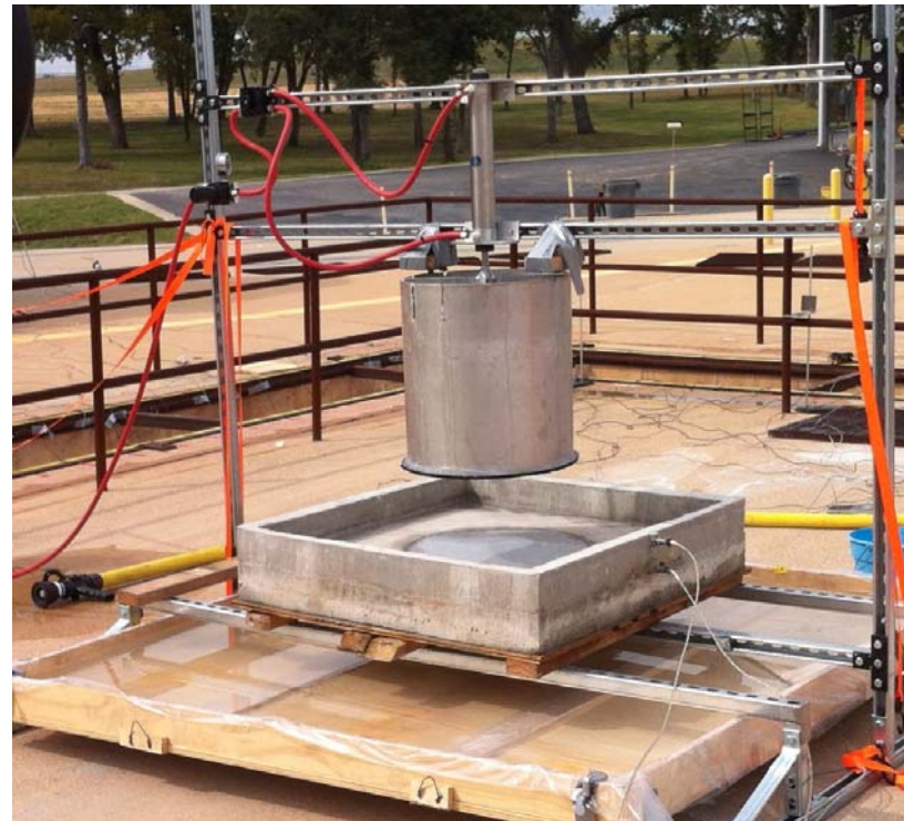
Setup of bund overtopping test at Brayton Fire Training Field
